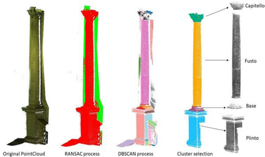
Figure 3 : Segmentation process for element selection
