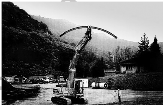
Figure 6.10 Clamp for setting steel ribs.
