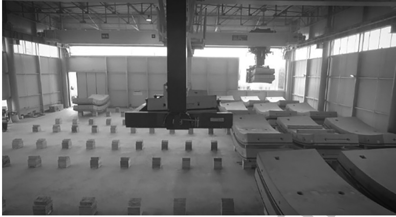
Figure 6.42 Pre-storage area and evacuation to storage area.
