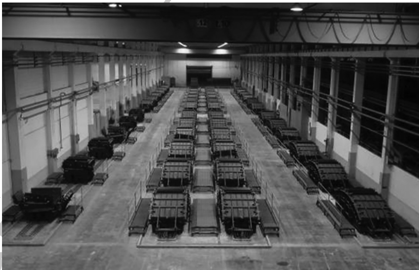
Figure 6.39 Stationary precasting line layout.
