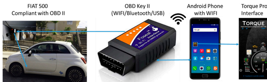
Figure 2. The trip data measuring scheme using OBD-key.
