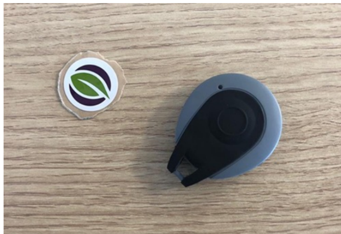
Fig. 2. adhesive NFC tag (on the left) to place in the field (Fig. 3) and portable gadget (on the right) assigned to each farmworker.
