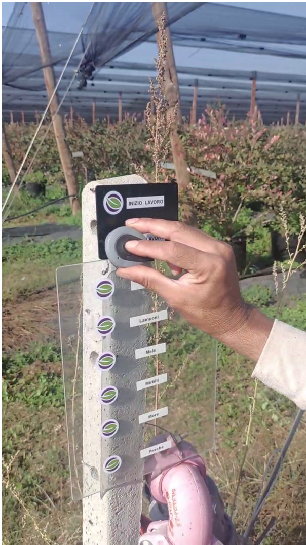
Fig. 3. Selection of a processing stage. Choosing a processing phase involves the farmworker positioning their smart device adjacent to the "start phase" tag, followed by placing it near the specific job description (harvesting, pruning, etc.). Upon completing the work, the farmworker positions the device near the "finish phase" label.
