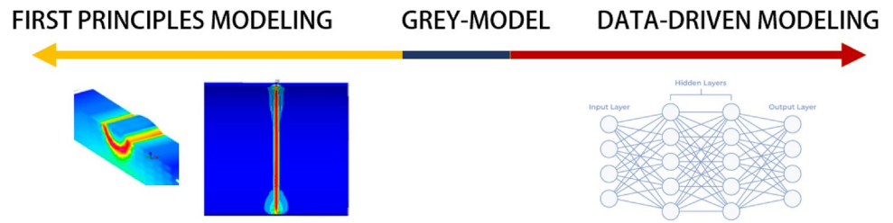
Fig. 4 Physics-based models in which 3D geometry and first principles are used and data-driven modelling techniques may be employed to develop virtual replica of physical assets
