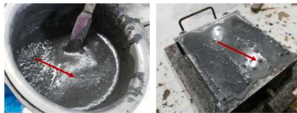
Fig. 7. Fresh GNP-based mixtures (GNP7): segregation (left) and bleeding with high content of air bubbles (right).
