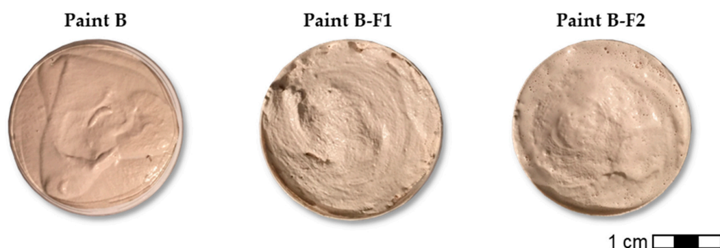
Figure 2. Aspect of Paint B after and before the addition of fillers.
