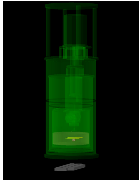
FIG. 10. The GEANT4 GUI output of Sim 4. It includes the ADR, the 30-mK plate, the magnetic shield, the copper box housing the TES substrates, and, in gray, the three sabers below the refrigerator.
