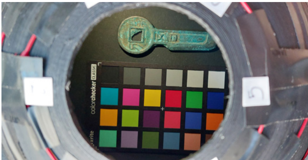
Fig. 3.5 Top view of the dome from the apical camera aperture. Particular of the acquisition of a sample with the reference to balance the final colour.
