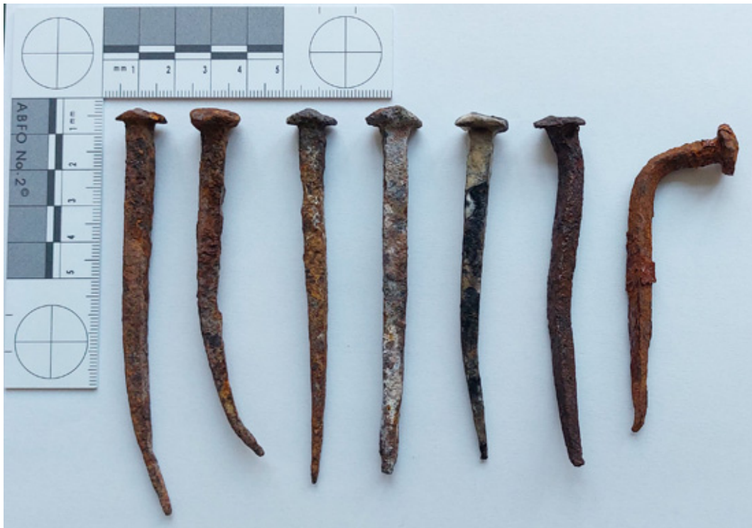
Fig. 4.7 Iron nails used to test the long-term protective effectiveness.
