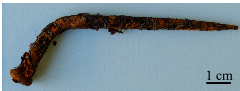
Fig. 4.8 Sample CH-15 treated with acrylates and then exposed to constant humidity chamber.
