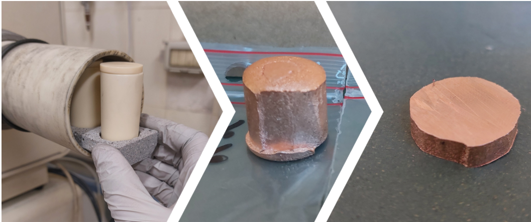
Fig. 2.7 Preparation of Cu-based reference samples: from the left, alumina cylindrical crucibles before being put in the tube furnace, example of obtained ingots and lastly, the sample after precise cutting.
