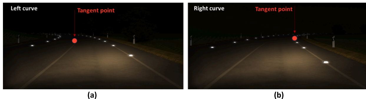
Fig. 1. Road stud layout adopted in Portera et al. (2023). Assuming the tangent point mechanism is used (Land & Lee, 1994), in the case of a left turn (a) the gaze is directed toward a road sign without LED studs, which is in contrast with the case for a right turn (b).
