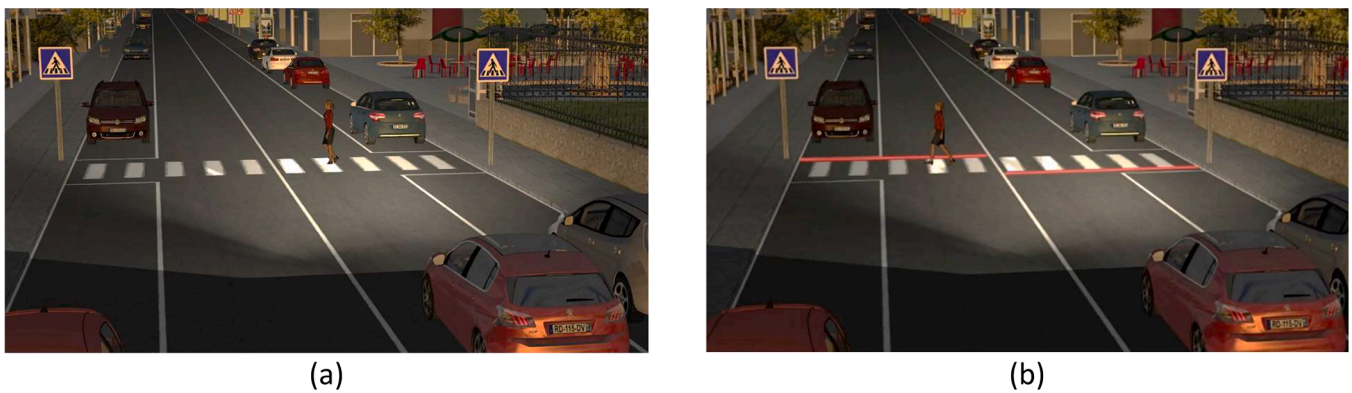
Fig. 2. (a) Conventional, and (b) smart mid-block crosswalks. In the smart crosswalk, the red LED light is activated when the pedestrian steps onto the crossing area.
