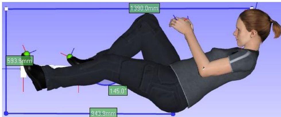
Figure 3 The 5 th percentile female dummy with the encumbrance dimensions in the sagittal plane.
