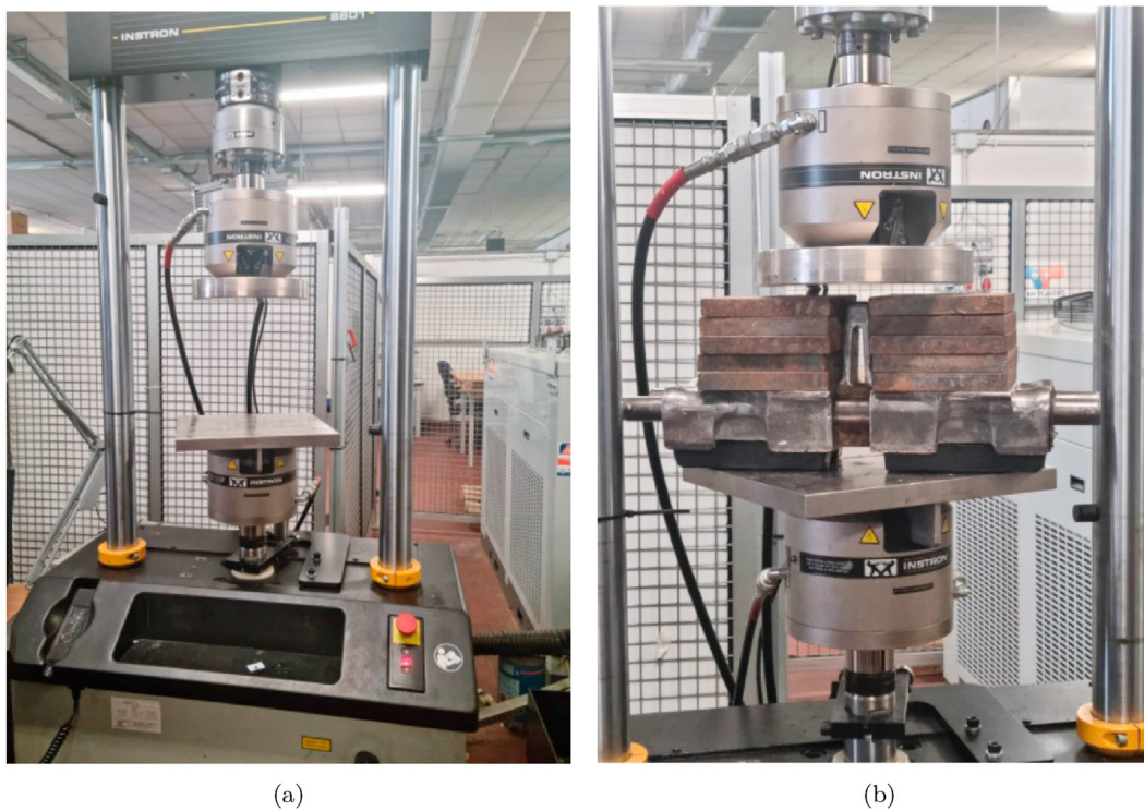
Fig. 4. Instron machine (a) for experimental characterisation of the track assembly component (b).
