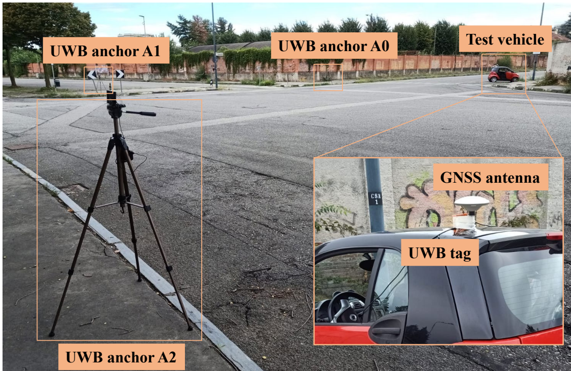
Fig. 6.10 Snapshot of the experimental scenario for the real-world test campaign. The deployed network of static UWB anchors is shown. Moreover, the UWB tag and the GNSS antenna on the road vehicle's roof are highlighted.
