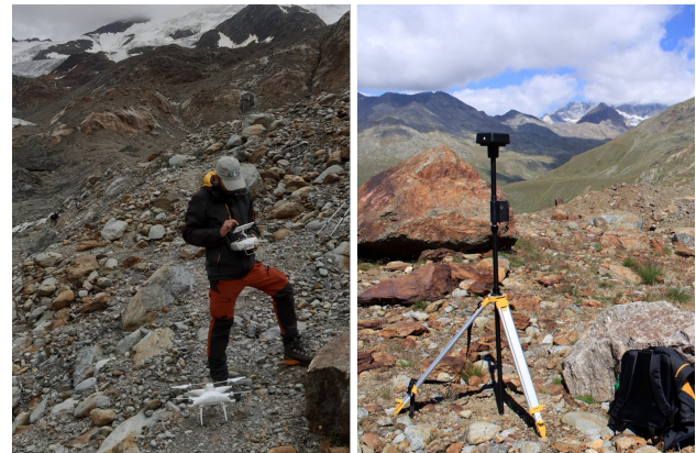
Figure 1. DJI Phantom 4 RTK and D-RTK 2 high precision GNSS mobile station.
