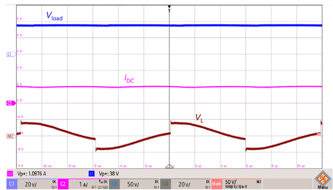
FIGURE 13 Measurements of the load voltage (blue), DC magnetizing current (magenta), and voltage drop over the AC winding of the auxiliary inductor (red), when the DC magnetizing current is set to 1 A and the transferred power is approximately equal to 30 W.
