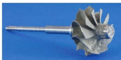
Figure 4: Assembly of machined SEB-PBF turbocharger wheel and shaft. Machining was realized for double hexagon head, radius of turbine blades as well as back face. The assembling between shaft and turbocharger wheel was performed by brazing[13]
