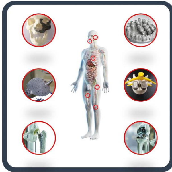
Figure 6: Schematic diagram of the biomedical application of additive manufacturing of bio metals includes cranial prosthesis, dental implants, acetabular cup, interbody fusion cage, hip prosthesis and knee prosthesis. [12]
