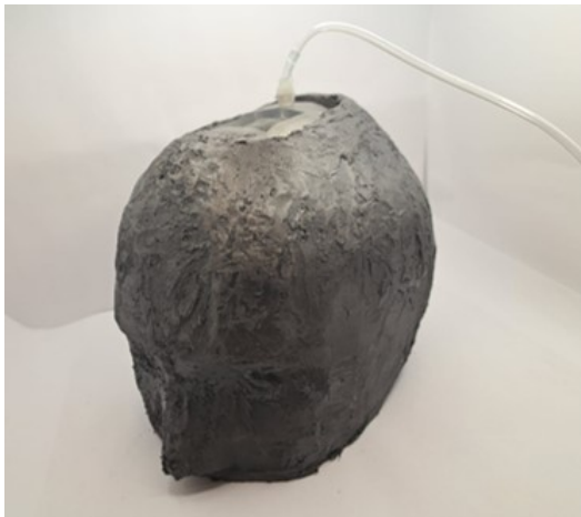
Fig. 2: Multi-tissue head phantom.
