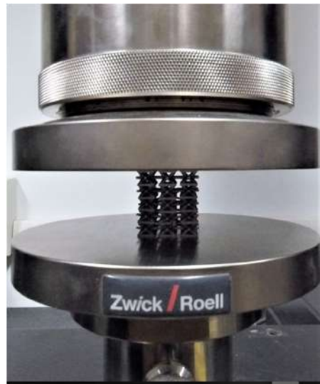
Figure 3. Setup of the Zwick Roell machine for uniaxial compression test on trabecular specimens.
