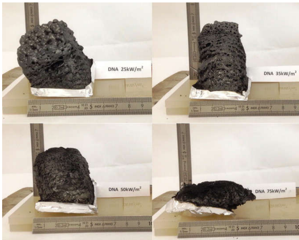
Figure 7. Intumescent features of DNA, as assessed through cone calorimetry tests performed at different irradiative heat fluxes (from 25 to 75 kW/m 2 ). Reprinted with permission from [46]. Copyright Elsevier, 2014.
