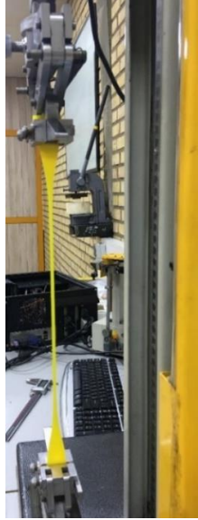
Fig 3. Uniaxial tension loading test [14]
