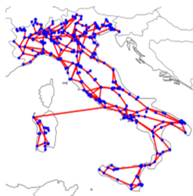
Figure 2. 339-bus simplified Italian transmission network (179 lines at 220 kV and 233 lines at 380 kV).
