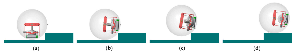
Figure 19. Four frames of the simulation of the robot overcoming a step of 100 mm.
