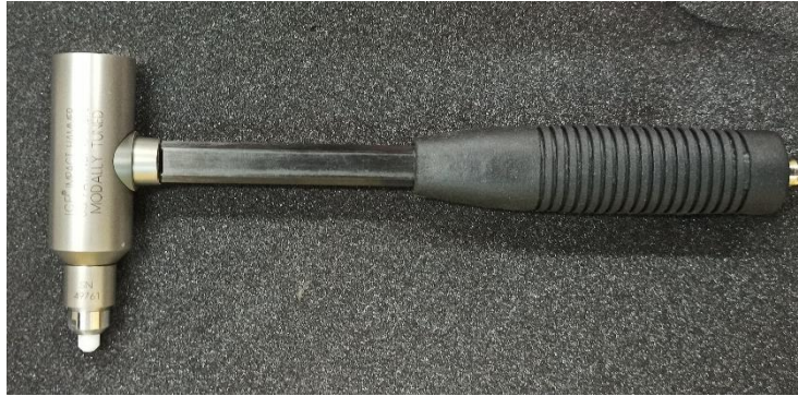
Figure 34. Impact hammer adopted to characterize the force profile.
