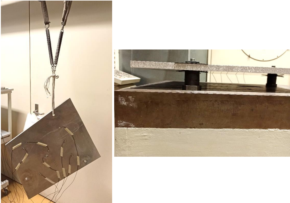
Figure 56. Configurations with free (on the left) and fixed (on the right) boundary conditions.
