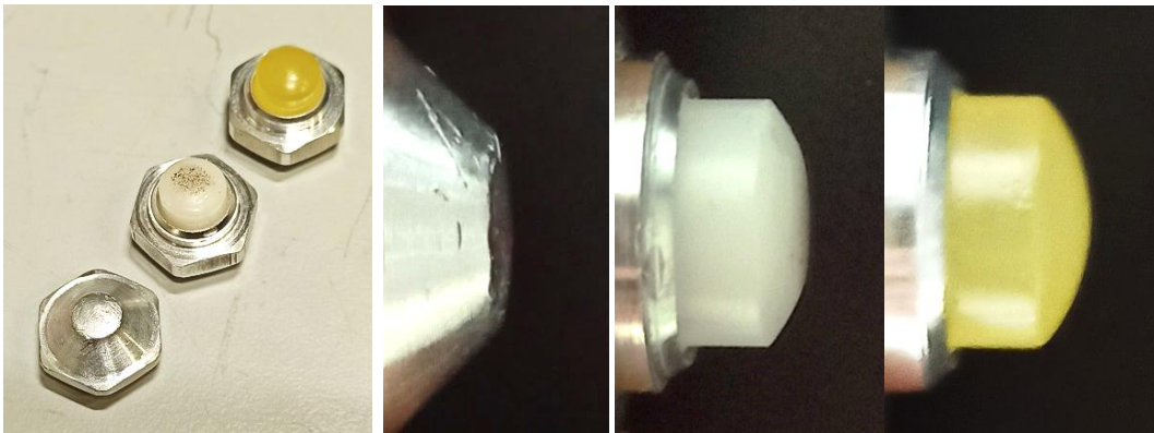
Figure 53. From left to right: impact tips adopted during the tests; side views with a focus on the curvature radius of the impact tips in aluminum, Delrin, and Polyurethane.
