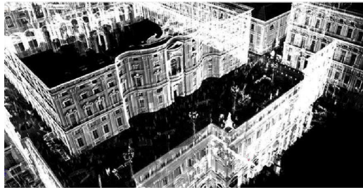
Fig. 4. Registered point cloud [44].
