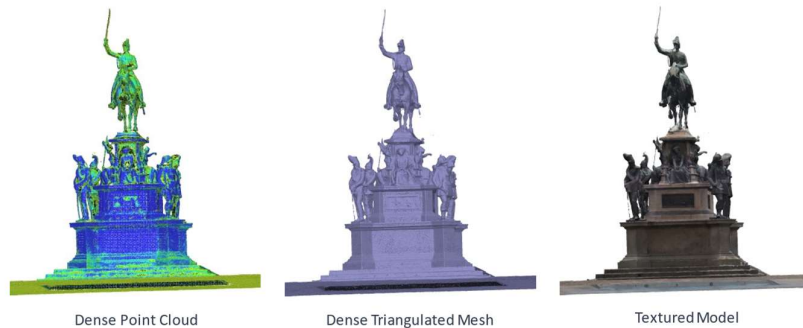
Fig. 5. Dense point cloud (left), dense triangulated mesh (middle) and textured model (right) of Carlo Alberto's statue.
