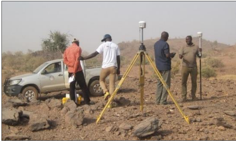
Fig. 3. Environmental conditions during the survey activities in the field. The master receiver (on the tripod) is in the foreground, while the rover receiver is in the background.
