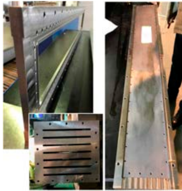
Figure 8. Modular PAV prototype made of vanadium.
