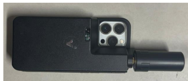
Figure 1. iPhone 15 Pro with the viDoc RTK Rover
