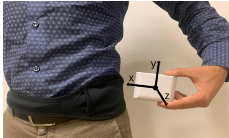
Figure 1. Wearable sensor (STAT-ON™) position and axes orientation.
