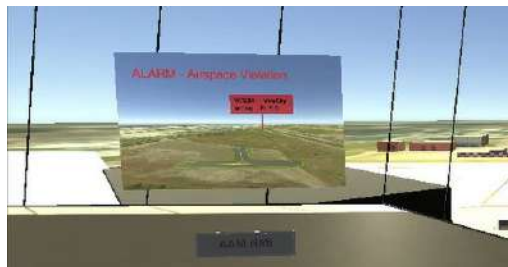
Figure 3 Safety net visualisation: a landing drone trespassing into a restricted area.
