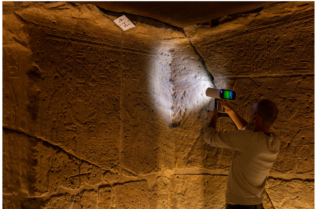
Figure 11. The SLS during the acquisition. The default scanning range of the Artec Leo is 0.35 to 1.2 m.
