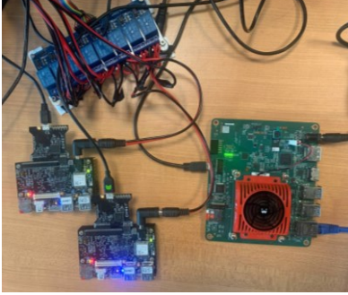
Fig. 2: Embedded Distributed Platform with three nodes.
