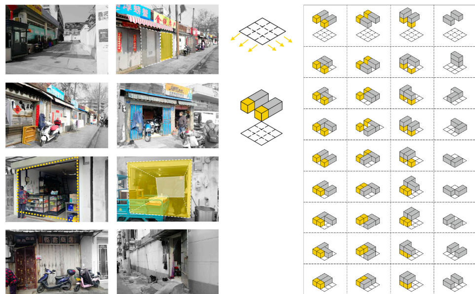
Figure 5. The co-optation of existing building types for new housing and micro-trading activities in Nanjing (Hehua Tang area): in yellow the new small shops, in grey residential spaces as legacy of the original courtyard-houses urban fabric. From the Design Studio “Urban morphology, architectural typology, contemporary settlement patterns” at SEUArch 2022 (Professors Bao Li and Marco Trisciuglio).
