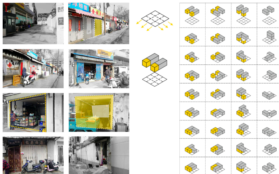
Figure 5. The co-optation of existing building types for new housing and micro-trading activities in Nanjing (Hehua Tang area): in yellow the new small shops, in grey residential spaces as legacy of the original courtyard-houses urban fabric. From the Design Studio “Urban morphology, architectural typology, contemporary settlement patterns” at SEUArch 2022 (Professors Bao Li and Marco Trisciuglio).
