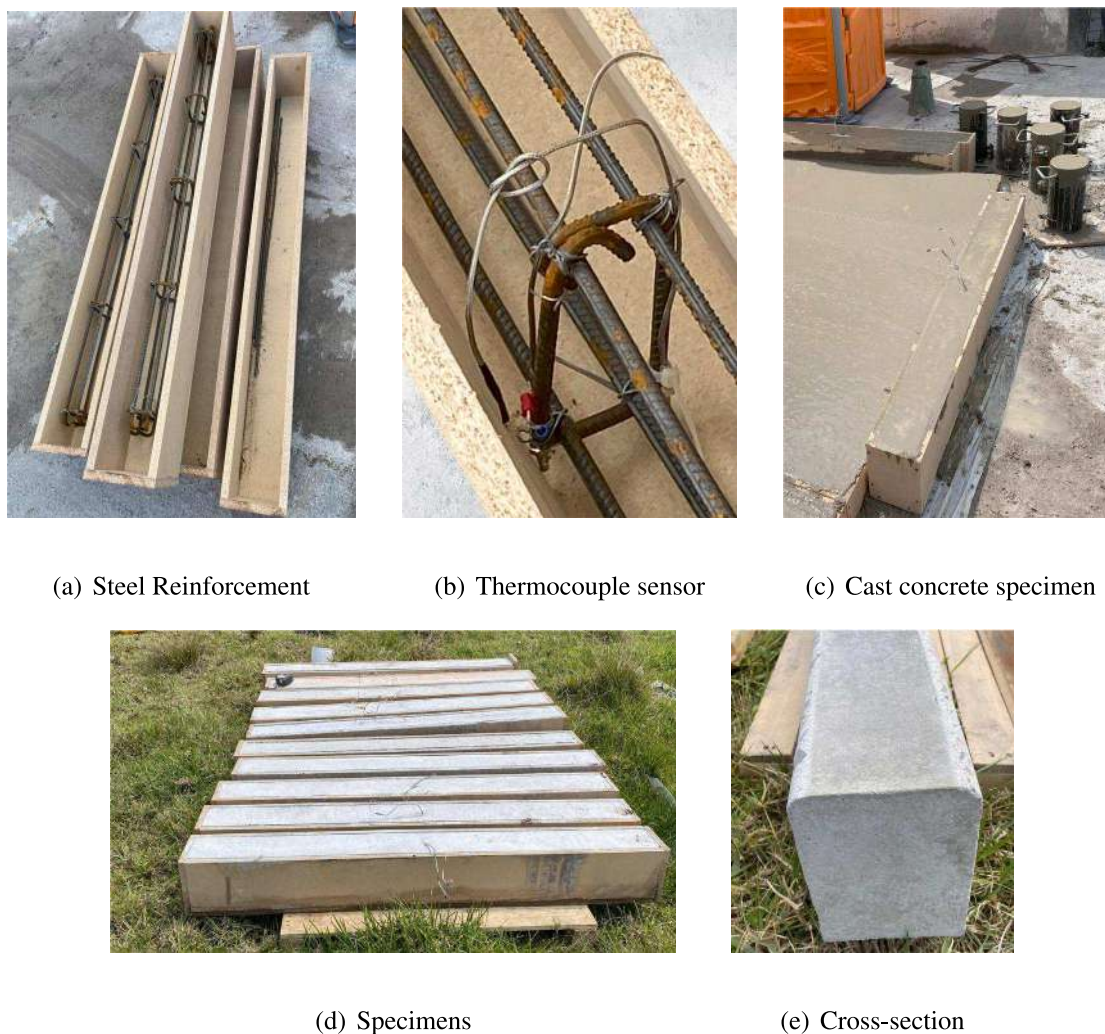
Fig. 1. Specimen fabrication process.
