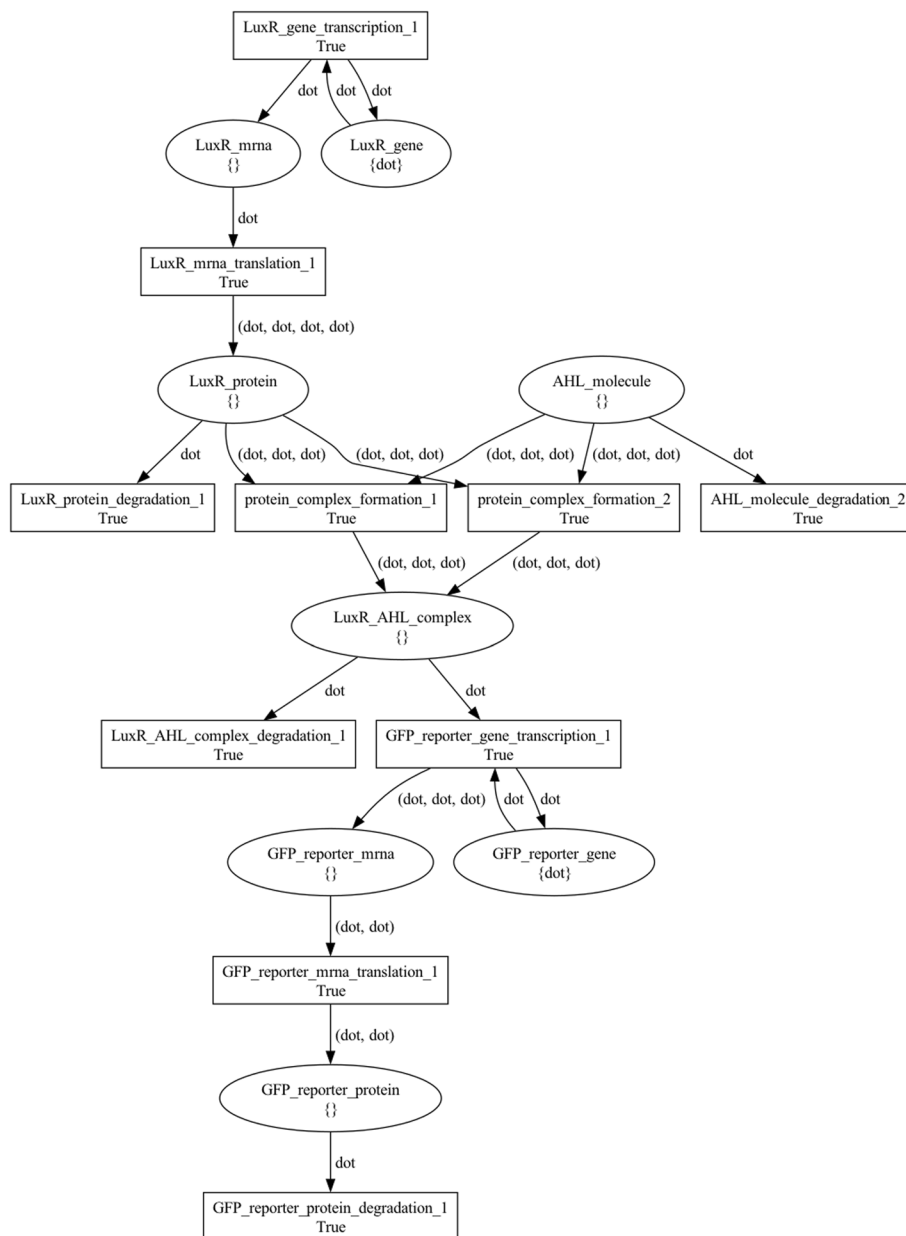
Fig. 7 The sensor bacterial_consortium net token architecture. Places model genes, transcripts, proteins, and molecules, while transitions model processes involving them, such as transcription, translation, degradation, and enzymatic reactions. Black tokens model discrete quantities of resources in each place and are represented by the dot symbol
