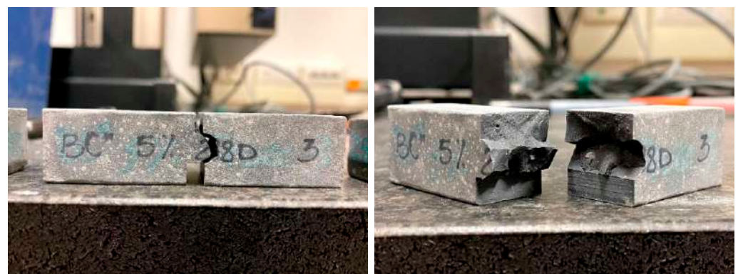
Figure 12. Tortuous crack path and rough fracture surface. B 5% at 28 days.
