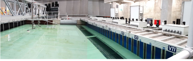
Fig. 3: Photograph of the physical wave tank. Waves are generated with 30 wave paddles.
