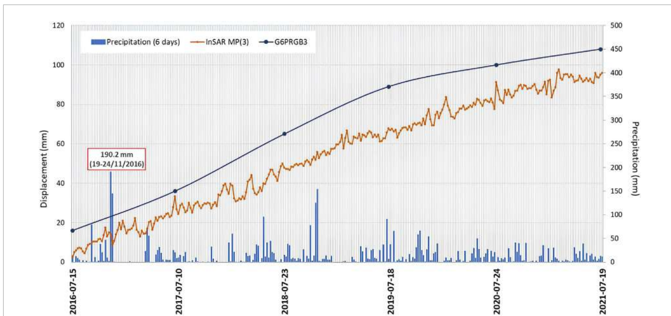
FIGURE 13 Displacements time series at the top of landslide in Pragelato.
