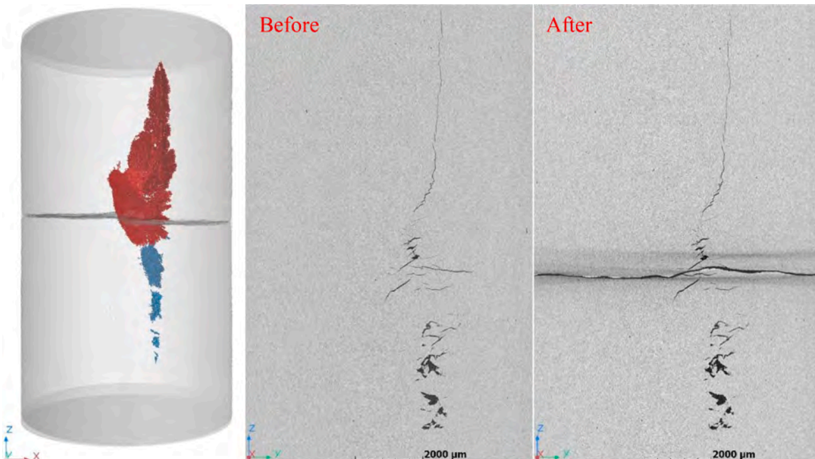
Fig. 11. Illustration of alumina specimen 8 cracks.
