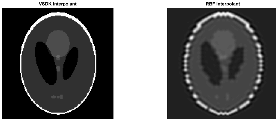
Fig. 3: Reconstruction of the Shepp-Logan phantom for given sampling data at the nodes \mathbf{LS}_2^{(40,41)} using the VSDK scheme (left) and the RBF interpolation (right). For both schemes, the C^2 -Matérn kernel is used. In the VSDK scheme, the scaling function \psi is a priori known.
