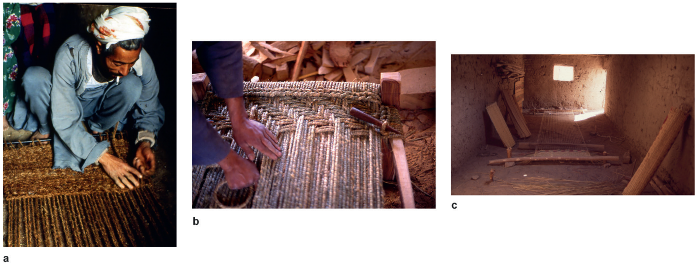
Fig. 8 – Matting looms (photos W. Wendrich). a. Mat-maker Amrit in el-Amariyya (Egypt) making a twined mat on a simple loom; b. Bed frame in which the warp is fastened first, after which the weft is woven in Daraw (Egypt); c. Matting workshop with a horizontal ground loom with heavy beater beam, cotton string warp and a weft of individual plant stems (rushes), Dakhla Oasis (Egypt).
