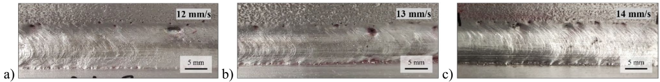
Fig. 3 Visual appearance of each sheet/cast GMAW joints carried out with a travel speed of a 12 \text{ mm/s} , b 13 \text{ mm/s} and c 14 \text{ mm/s}
