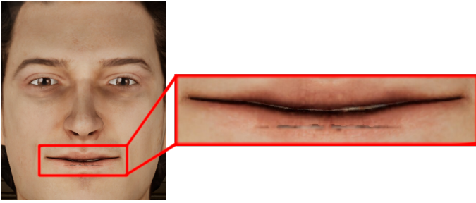
Fig. 2: Examples of visual artifacts on a Rocketbox character rendered with all AUs’ weights to 1.
