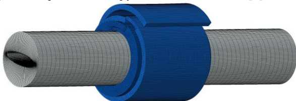
Figure 1: Cuff model (in blue), designed by thickness of 2 mm and length of 17 mm, in interaction with the urethral model (in grey).
