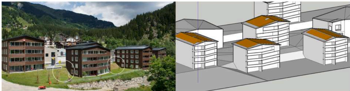
Fig. 6. Building and ground modeling - detail from the case study. Adapted from Dacos, (2017).
