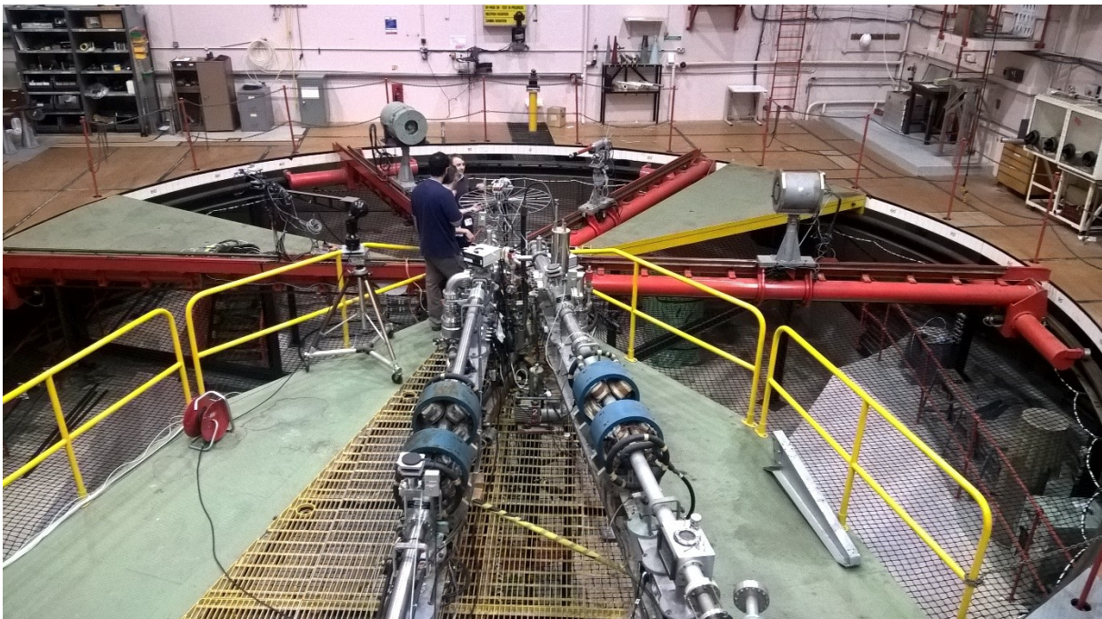
95 Fig. 1 Experimental hall inside the Chadwick facility. The NG is located in the centre of the hall. The two long 96 counters and the NE-213 scintillator are situated above the red rails in the centre of the above image.
