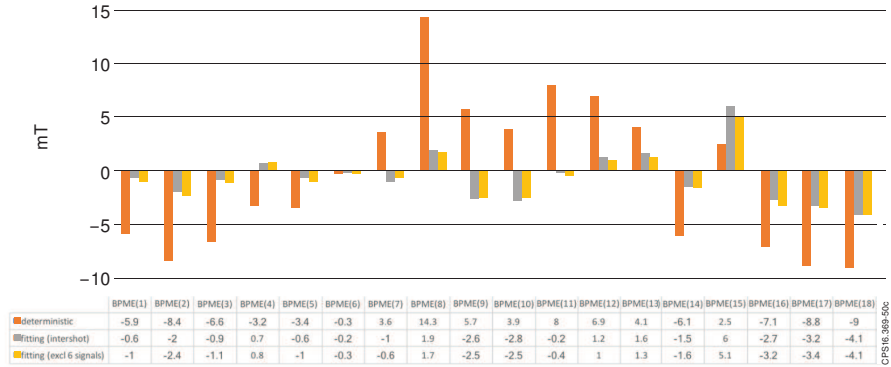
Figure 27: Poloidal probes signals for JET discharge 91576 at t=55.028s during the flat-top. The plot shows EFIT++ calculated signals with measurements subtracted. (i) ■ deterministic model configured with the standard JET intershot settings but excluding 4 flux loops and 2 saddle loops; (ii) ■ fitting iron model with the same magnetic measurements as for case (i); (iii) ■ fitting model configured with the standard JET intershot settings;
