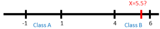
Fig. 1: Given the training set \{(-1, A), (1, A), (4, B), (6, B)\} , predict the class and probability interval of x=5.5 with the nearest centroid taxonomy (NCT).
