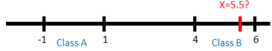
Fig. 1: Given the training set \{(-1, A), (1, A), (4, B), (6, B)\} , predict the class and probability interval of x=5.5 with the nearest centroid taxonomy (NCT).
