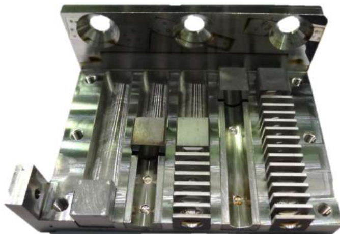
Fig. 2. Five-way cassette from main chamber wall. From the left: mirror at 0.0 cm at the cassette mouth placed in the standard square channel; 1.5 cm deep circular and baffled channels and a similar set with mirrors at the depth of 4.5 cm.
