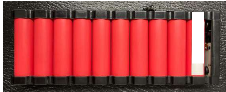
Figure 18. 25 Ah battery pack module.
