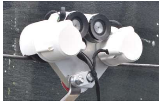
Figure 24. Trolley traction structure with 3D-printed cover.
